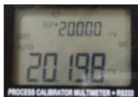
IN/OUT CHECK CLOSE: 4mA, OPEN: 20mA
