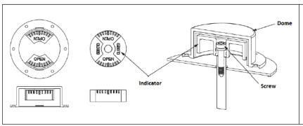
The position of the valve is indicated by the indicator. If its alignment is incorrect, remove the cover and proceed to its setting by unscrewing the attachment screw.
